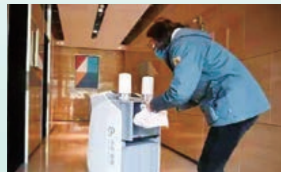
◆ Shanghai Henderson CIFI Center The robot can take the elevator autonomously and call the front desk to inform the customer to pick up the meal. The robot has its own smoke disinfection function, which can carry out full-automatic disinfection.
